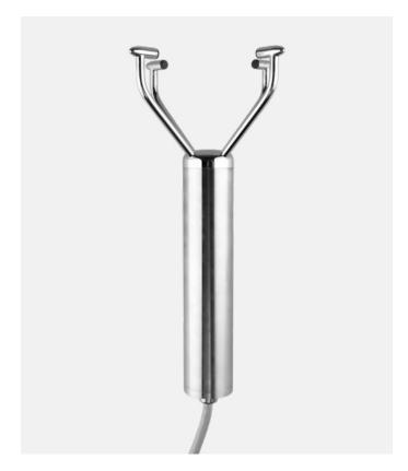
The sensor combines the latest patented advances in ultrasonic technology. The elimination of moving parts, together with a rugged stainless steel construction means that the WindObserver II is virtually maintenance free and requires no calibration on site. The heated head keeps the unit free from ice and snow, providing continuous use even in the most extreme weather conditions.
