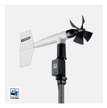
The wind speed sensor is a four blade helicoid propeller. Propeller rotation produces an AC sine wave voltage signal. The wind direction sensor is a rugged yet lightweight vane. Vane angle is sensed by a precision potentiometer.
