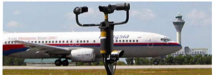
VPF sensors were the first forward scatter sensors to be used in a UK CAA approved RVR system on a CAT III runway.
