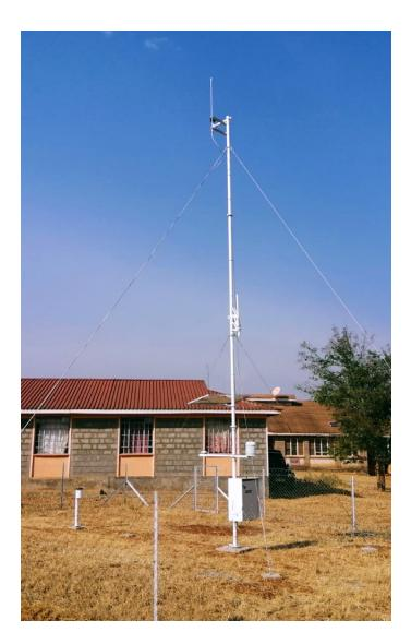
The superstrong MM10-100 is usable in winds up to 100 m/s and provides a stable platform for measuring equipment. Both MM10-75 and MM10-100 are easily installed by three persons.
