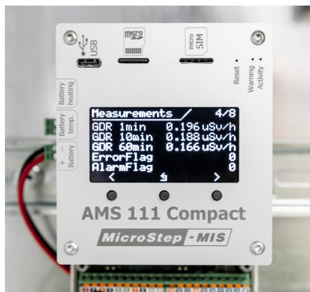
RPSG-07 mounted on a solar powered Gamma Dose Rate station with a precipitation detector and AMS 111 Compact data logger.
