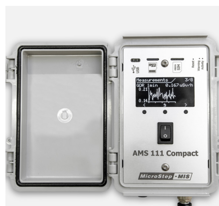
RPSG-07 mounted on a solar powered Gamma Dose Rate station with a precipitation detector and AMS 111 Compact data logger.
