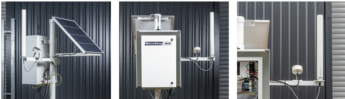
RPSG-07 mounted on a solar powered Gamma Dose Rate station with a precipitation detector and AMS 111 Compact data logger.
