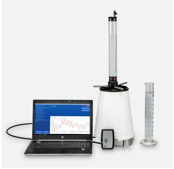
RGcal is an electronic impulse counter, that counts the tips of a tipping bucket rain gauge and measures the time between the overturning of a bucket. The information is sent to the PC via standard USB.
