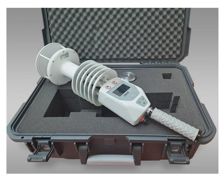
With a professional data logger included, the handheld station is suitable not only for short-period measurement but also for longer campaigns. In addition to SD-card and USB-C, the station also provides a 4G modem and Bluetooth interfaces
