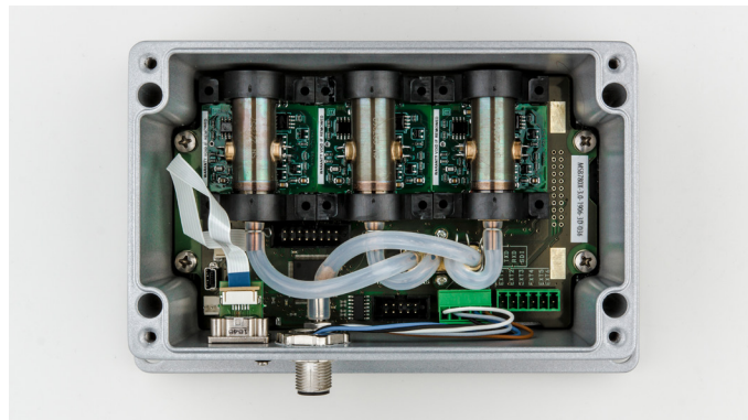
MSB780X can be equipped with three solid-state transducers for use in applications that require it.
