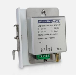
MSB181 can be ordered with one of the following output options: SSDI-12, RS-232, RS-485, or analog voltage ranging from 0 to 2.5 V. Supply current is less than 6 mA at 12 V. The version with SDI-12 features 50  $\mu$ A sleep mode. Time to first sample less than 1 s can be achieved with RS-485 and analog versions.
