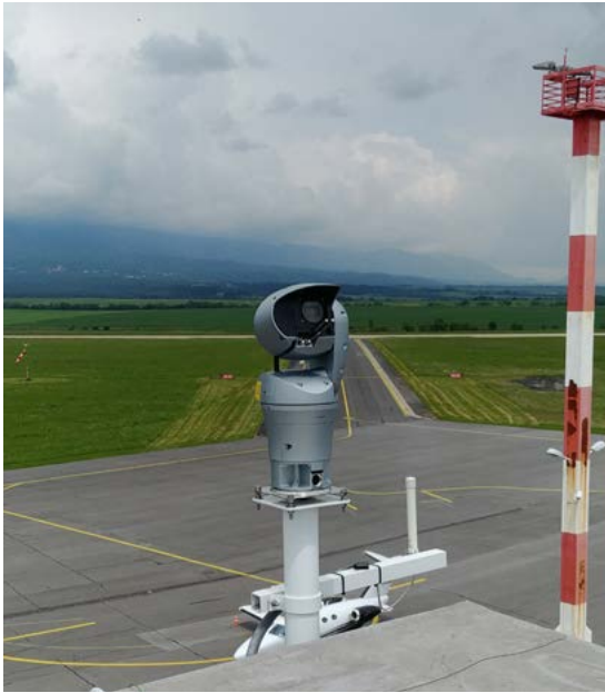
Examples of visual and infrared cameras with rotation enabled
