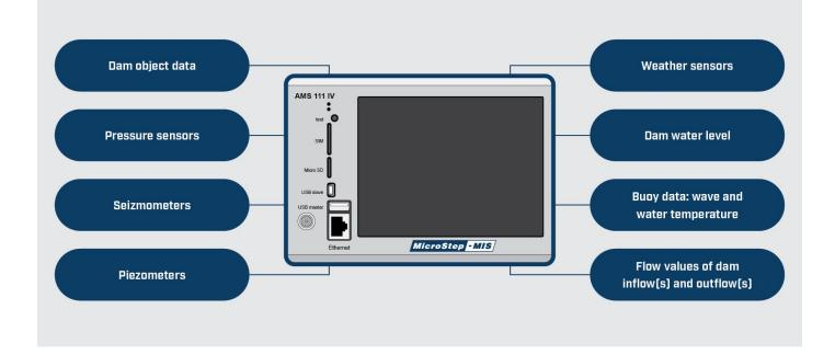
Collection and pre-processing of the measured data are ensured by the smart data logger. The optional collection system is the Data Logger AMS 111 IV.
