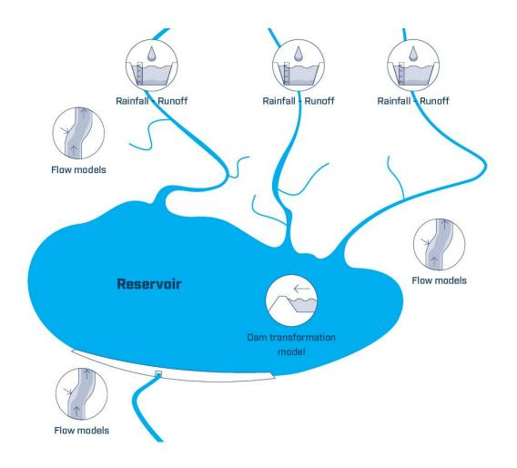
**Rainfall-runoff models** (HEC-HMS, HYPE, HBV) are transforming rainfall to a runoff a can be directly used for computing inflow to the dam. Models run in minute, hourly, or daily time steps, with the dependence on the needs of the dam operating authority.
