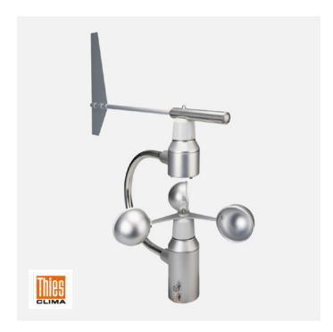
The wind speed is measured opto-electronically in contactfree and wear-resistant manner. It has an extremely low starting speed. The position of the wind vane is detected opto-electronically by a code disc.
