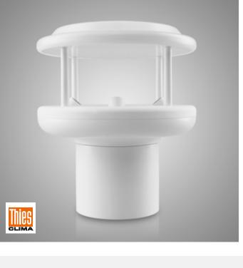
It measures wind velocity, wind direction, brightness, and precipitation. The wind velocity and wind direction are measured by an ultrasonic sensor in high-precision. The precipitation and its intensity are acquired via Doppler radar. A brightness sensor is included.
