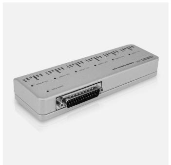
6 standard sensors, communicating over UART, SDI-12, or analog, can be connected to the Calibrator Extension Card. Using the RS-485 or RS-232 to the UART converter, almost all commercially sold devices can be connected to the card. The device supplies sensors up to 12 V.
