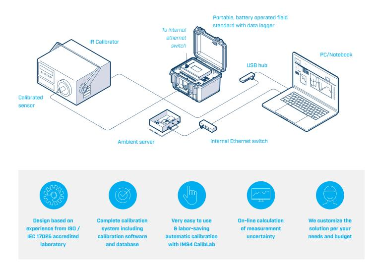
The calibration process is automated where possible. The software controls the infrared target temperature, takes readings from the reference, and values from the calibrated IR thermometer. The system allows calibration of instruments without electronic output too – the reading is taken and submitted into the system manually by an operator.
