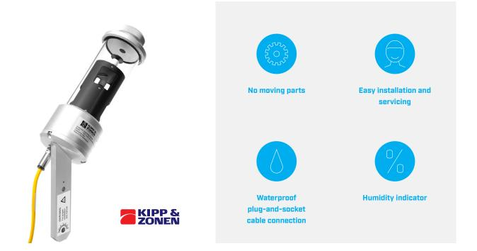
CSD 3 measures solar radiation through a high quality glass tube. It has no moving parts and uses 3 photo-diodes with specially designed diffusers to make an analogue calculation of when it is sunny. The output is switched high or low to indicate sunny or not sunny conditions. The calculated direct irradiance value is also available.
