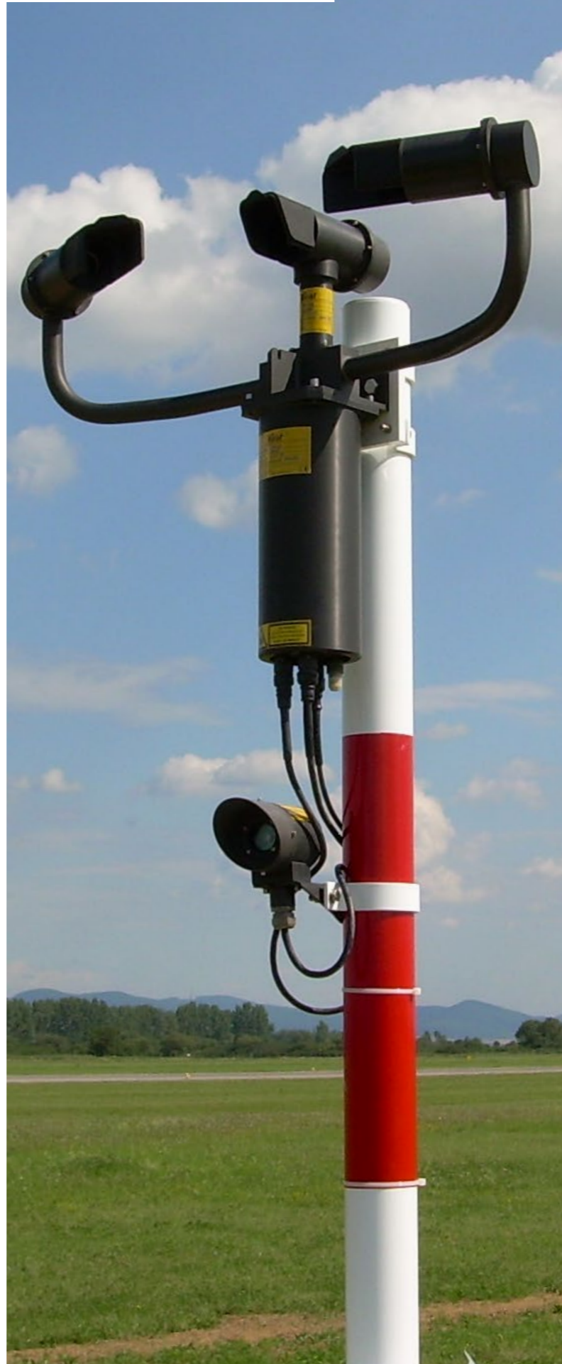
Forward Scatter Meter | VPF 700 series supplied by Biral
