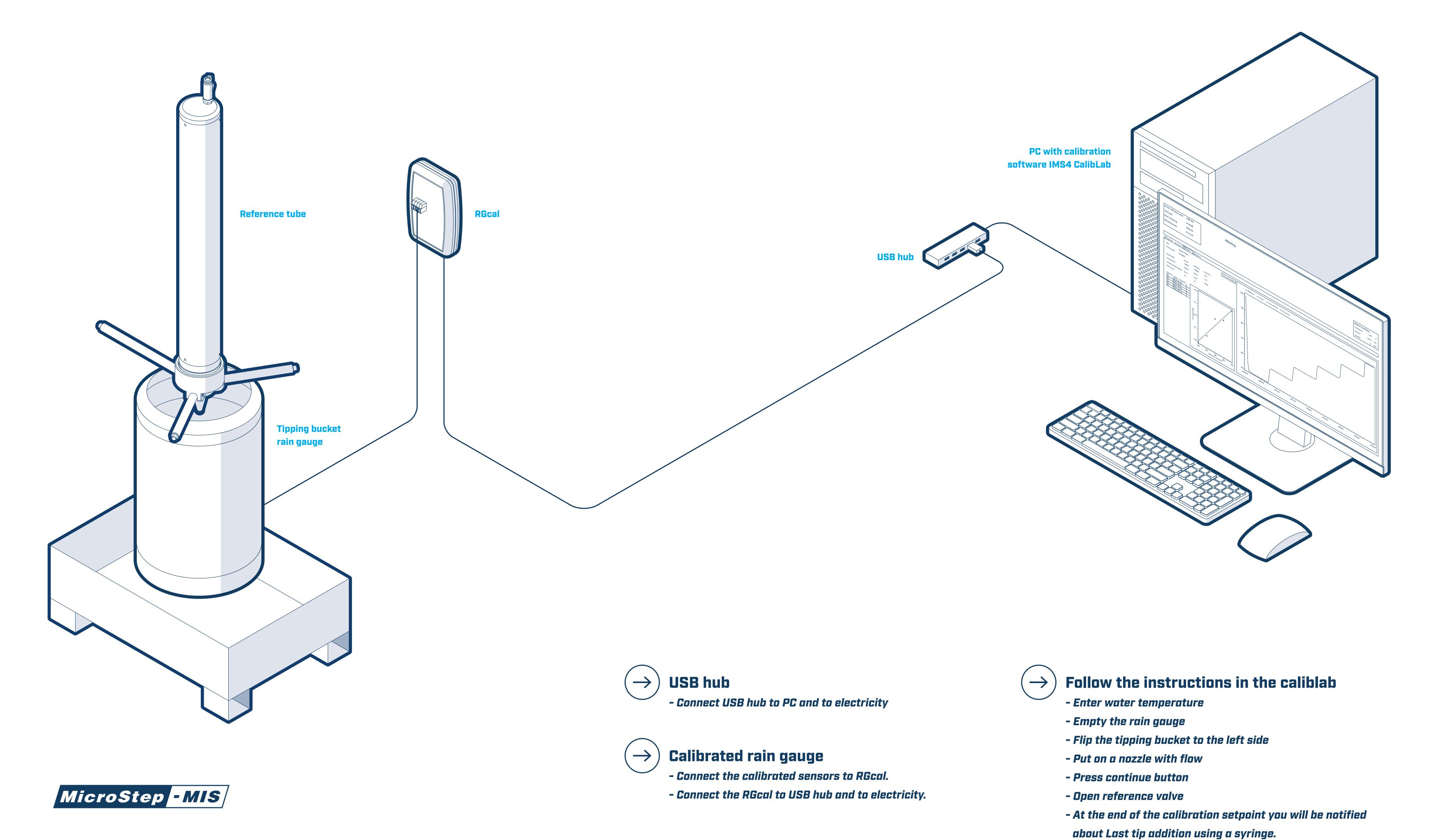
Calibration System for Tipping Bucket Rain Gauge
