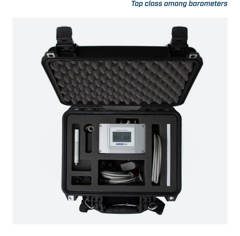
three versions (with 1, 2, and 3 transducers) of digital barometer MSB780X passed the tests successfully without any complaints. The measurement range was 500 – 1100 hPa with an error very close to the reference, the difference was 0.02 – 0.05 hPa. The employees of the testing facility were very surprised by the high level of accuracy of the device. The tests were carried out at fixed points with increasing and decreasing pressure in the entire measured range.
